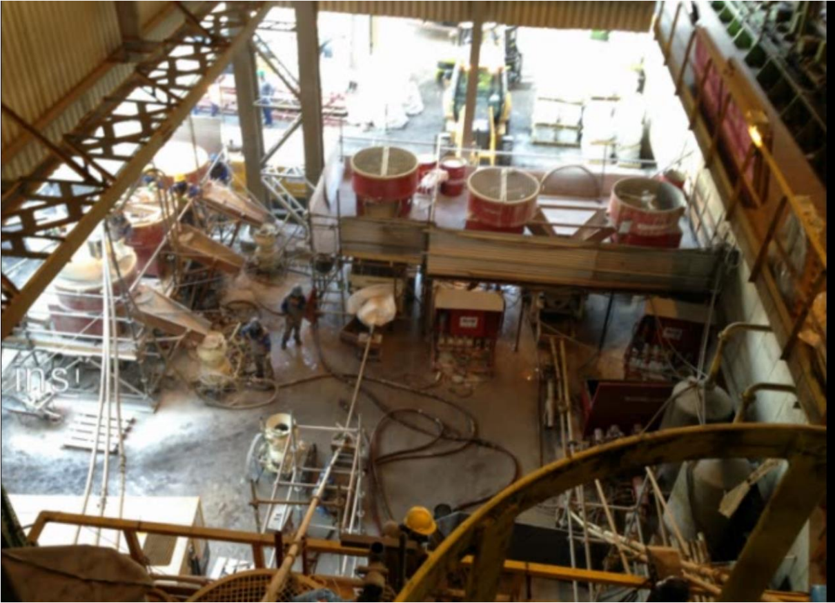
Left three Machine for prewetted gunning
