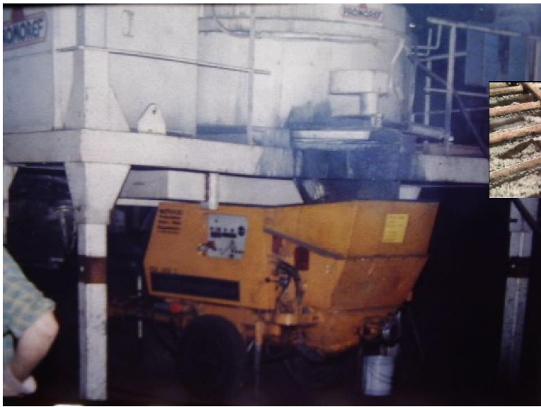
Sirma/Promoref 1992 with 5 ton mixer and first Putzmeister 2 cylinder Pump for ULC mix with SiC
